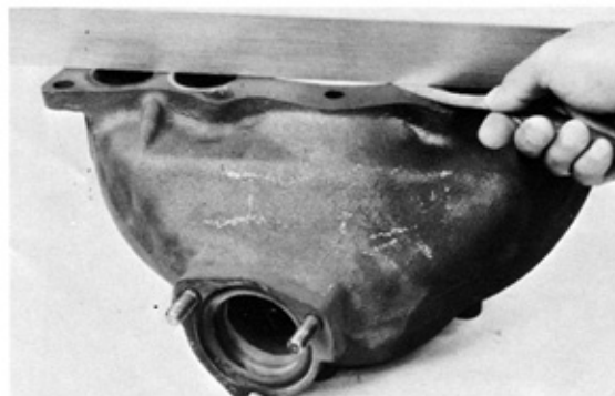
Fig. 7-9 Measure Manifold Warpage
