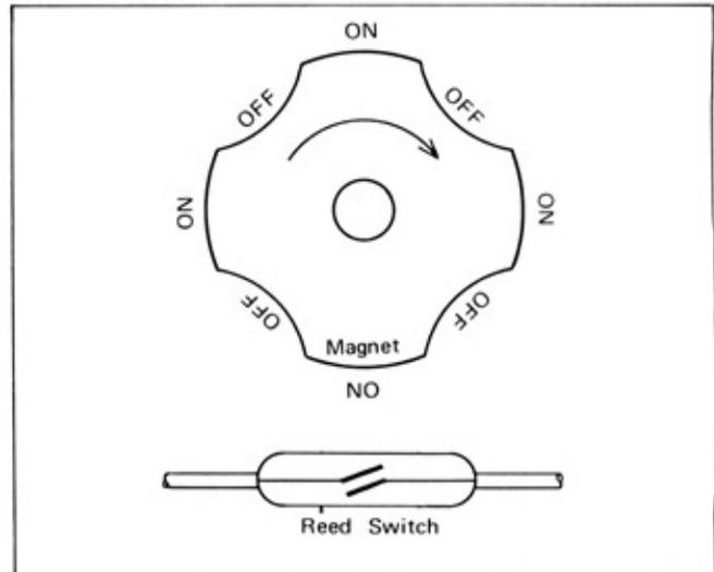
Fig. 1-2 Speed Sensor Operation
