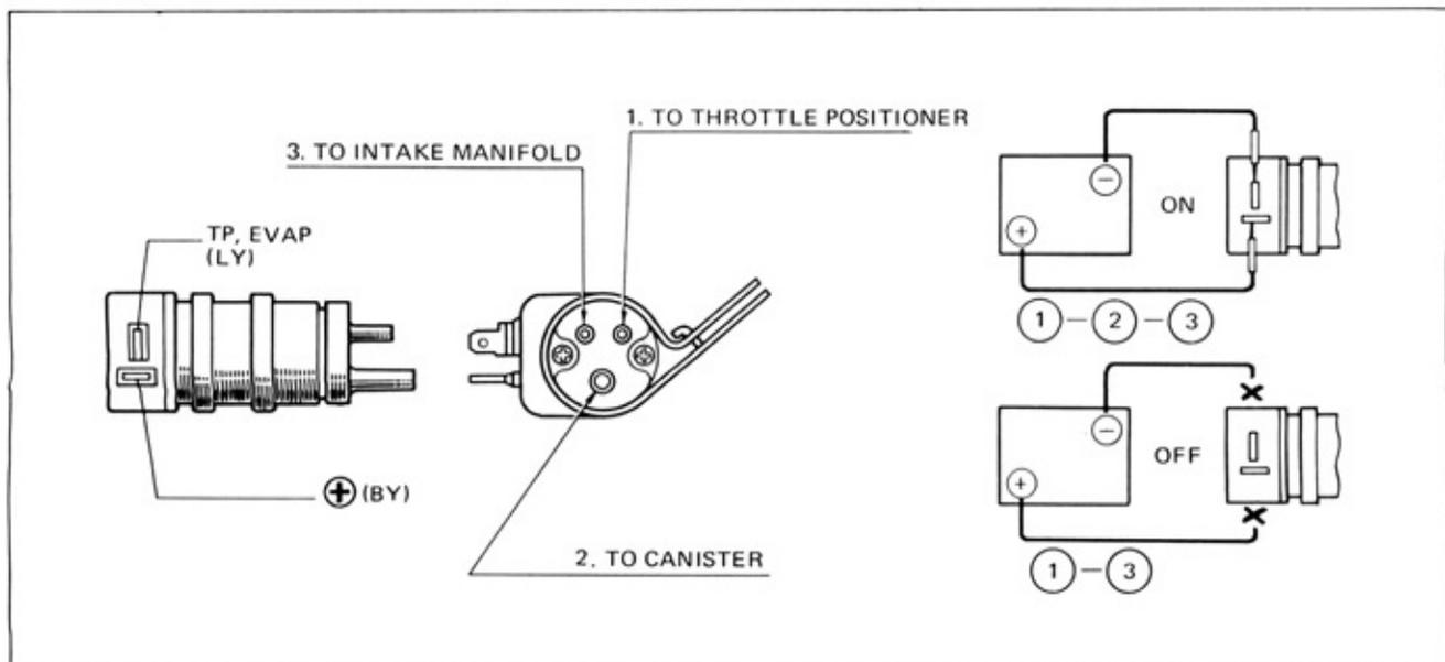
Fig. 1-17 Vacuum Passage Test (2T-C)
