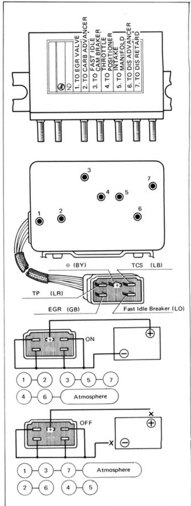
Fig. 1-21 Vacuum Passage Test
