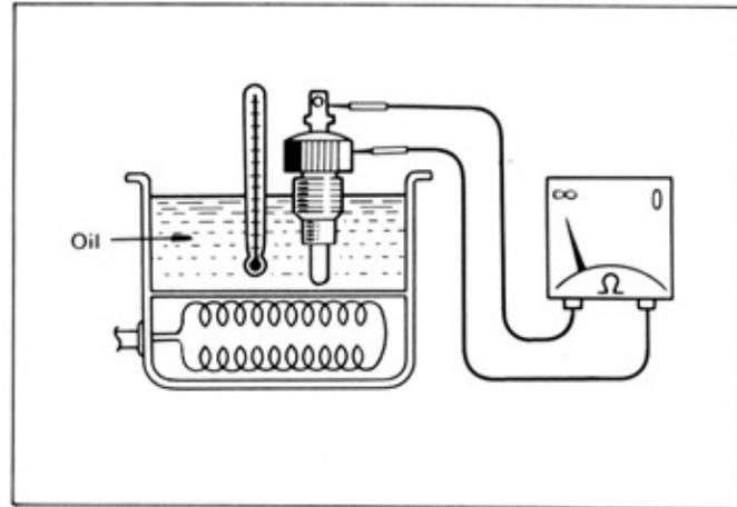
Fig. 1-10 Thermo Sensor Inspection
