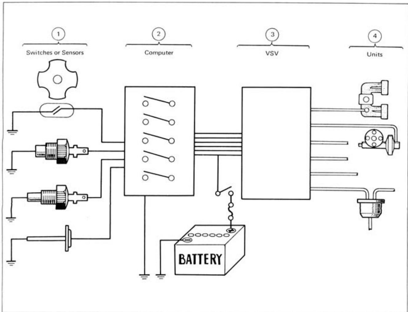
Fig. 1-1 Schematic Diagram of Parts Common to All Systems
