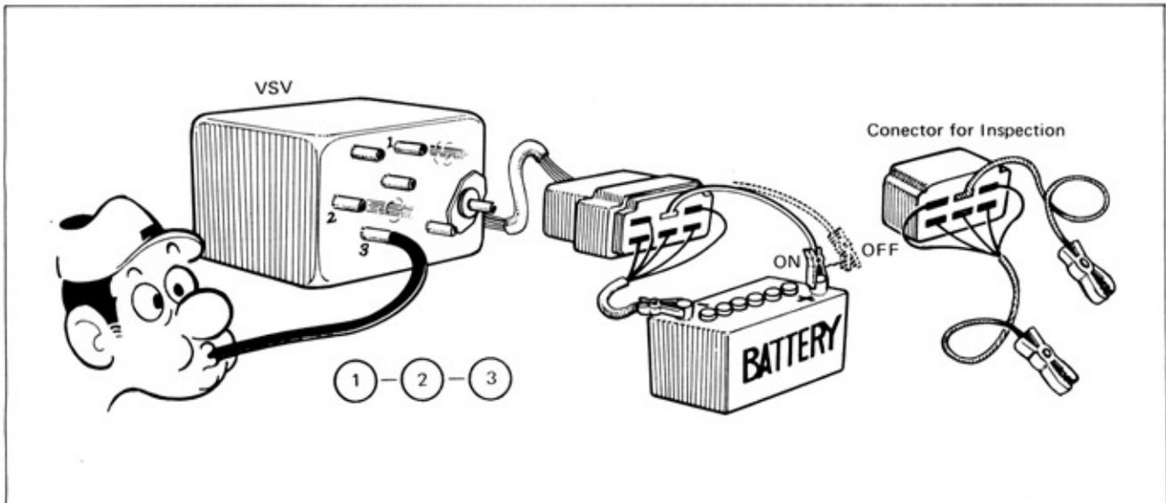
Fig. 1-16 VSV Vacuum Passage Continuity Test
