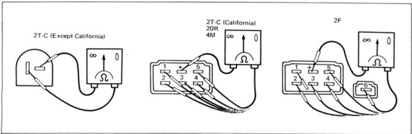
Fig. 1-15 Open-Circuit Test
