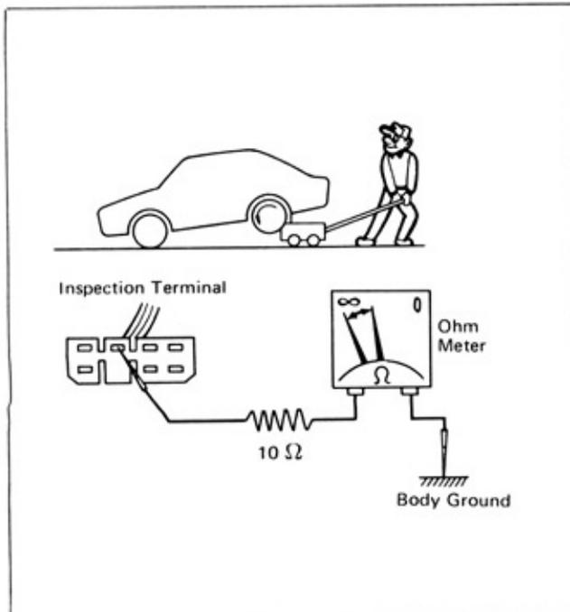
Fig. 1-8 Speed Sensor Inspection
