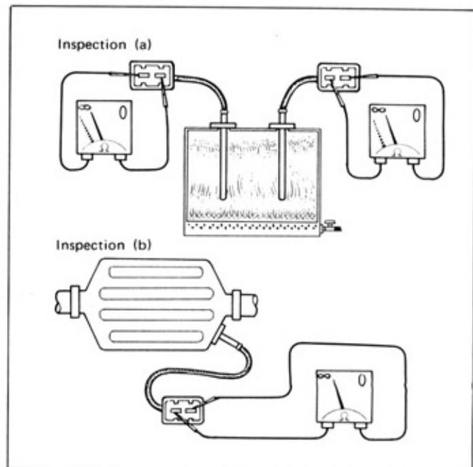
Fig. 1-11 Thermo Sensor Inspection
