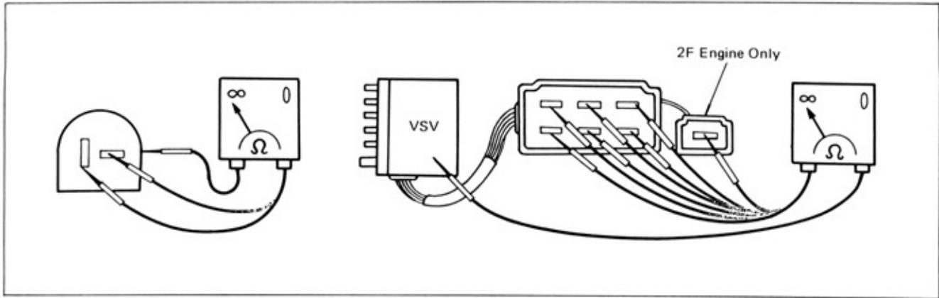
Fig. 1-14 Short-Circuit Test
