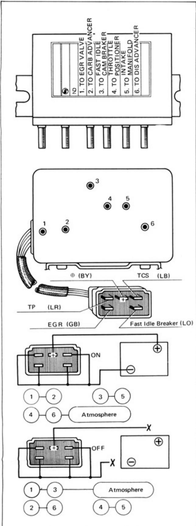
Fig. 1-20 Vacuum Passage Test (4M)
