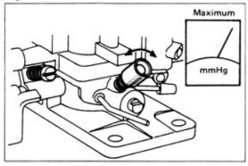
Set to maximum vacuum with the idle mixture adjusting screw.
