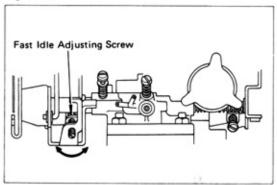
Insure that the engine is running at the specified rpm. If not, adjust with the fast idle adjusting screw.
