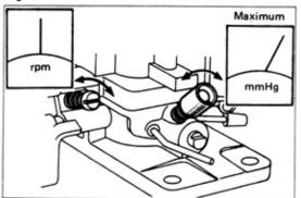
Repeat the above adjustments until the maximum vacuum and specified rpm is obtained.
