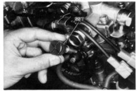
(3) If the concentration exceeds the specified value, tighten the idle mixture adjusting screw little by little until the concentration is within the specified value.
