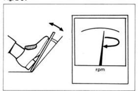
Check to see that the engine returns to idle when the accelerator pedal is released both suddenly and slowly.
