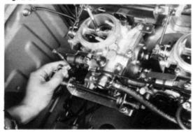
Connect the connecting rod so the idling rpm does not change. If it changes, adjust the rod length.
