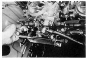
Disconnect front and rear carburetor the connecting rods.
