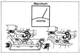
4 Adjust by turning each idle mixture adjusting screw so that intake manifold vacuum at the front and rear carburetors will be the maximum vacuum.
