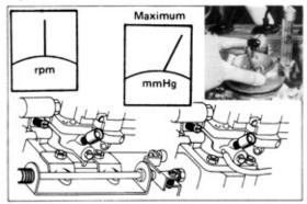
Recheck the intake manifold vacuum and intake air volume at the front and rear carburetors.
