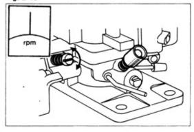
Set the idle with the idle speed adjusting screw.
