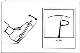
Race the engine momentarily by manipulating the accelerator link to verify that the engine will return to specified rpm when released.
