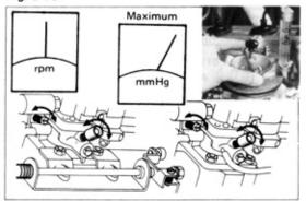
Repeat the above adjustments until the maximum vacuum, and intake air volume at the front and rear carburetors will be the same at specified idling speed.
