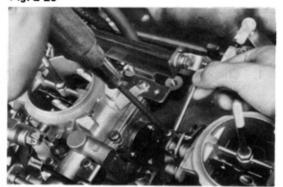
Adjust the link so that the front and rear carburetor choke valves open at the same time.
